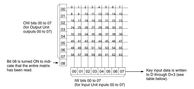
A selection signal is output to OW bits 00 to 07 consecutively for 3 cycles. Only one output bit will be turned on at a time. Bit 08 of OW is turned ON for 3 cycles after 07 to indicate when each round of reading the matrix has been completed.
